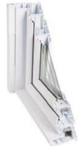
**TRIPLE GLAZING** - The glass package can be upgraded to a true 1 3/8" Triple-glazed Thermal Insulated Glass Unit, with three panes of glass, two LoE coatings, two Argon gas filled chambers and Super-spacer. The Triple Glazed Glass Package will minimize heat loss, boost indoor temperature stabilization and improve sound insulation.
